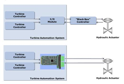
High Speed Controllers on I/O Eliminates External "Black Boxes"
