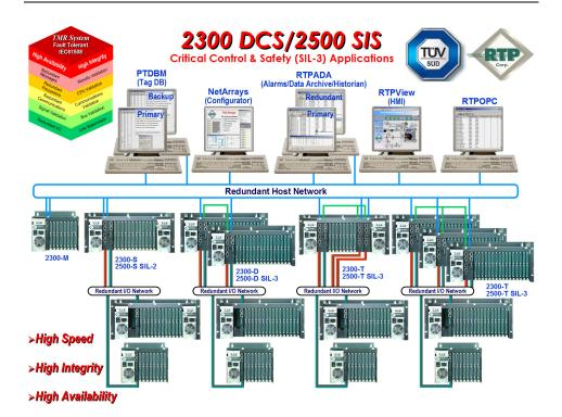
**RTP Automation Systems Offer Many Options for Redundancy**
